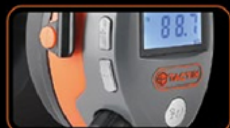
With listening mode (LIS) engaged, the ambient sound and conversations can be heard without removing the earmuffs
